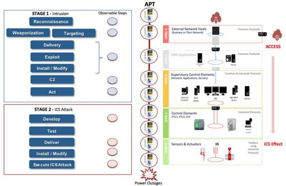
Figure 5: Ukraine Cyber Attack ICS Cyber Kill Chain and Purdue Model Mapping<sup>21</sup>
